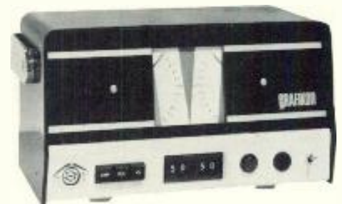
Electronic Color Analyzer for transferring color temperature readings from a master to other monitors. Digital pre-settable compensation for phosphor batches.
