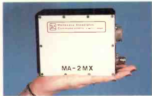
Dimensions: 4¾" x 2½" x 5¾", Weight: 3½ lbs. Power output: 12 watt, high stability 21-channel synthesizer, internal VSWR and thermal protection, dual audio channels.
