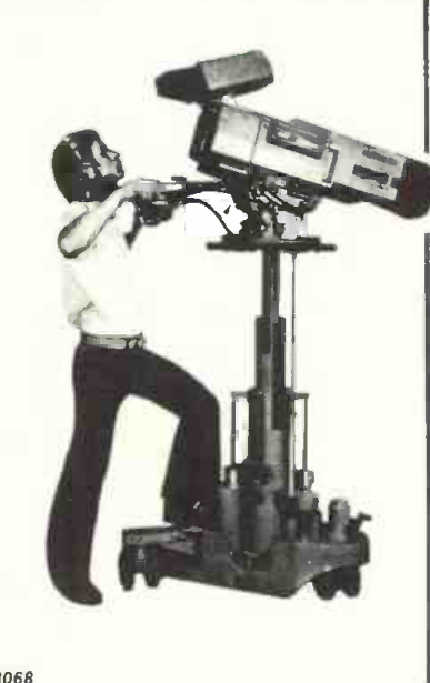
3068 THE PLOVER THREE STAGE TRANSPORTABLE PEDESTAL allows wide range elevation with a "break down" into two parts for easy transport. 50-200 lbs. can be counterbalanced without changing gas pressure with Vinten's multi-ram system.
