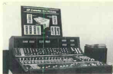
The modules that make up this API console from Datatronix can be fitted into a standard 19-inch rack in a variety of configurations suited to LPTV operations.
